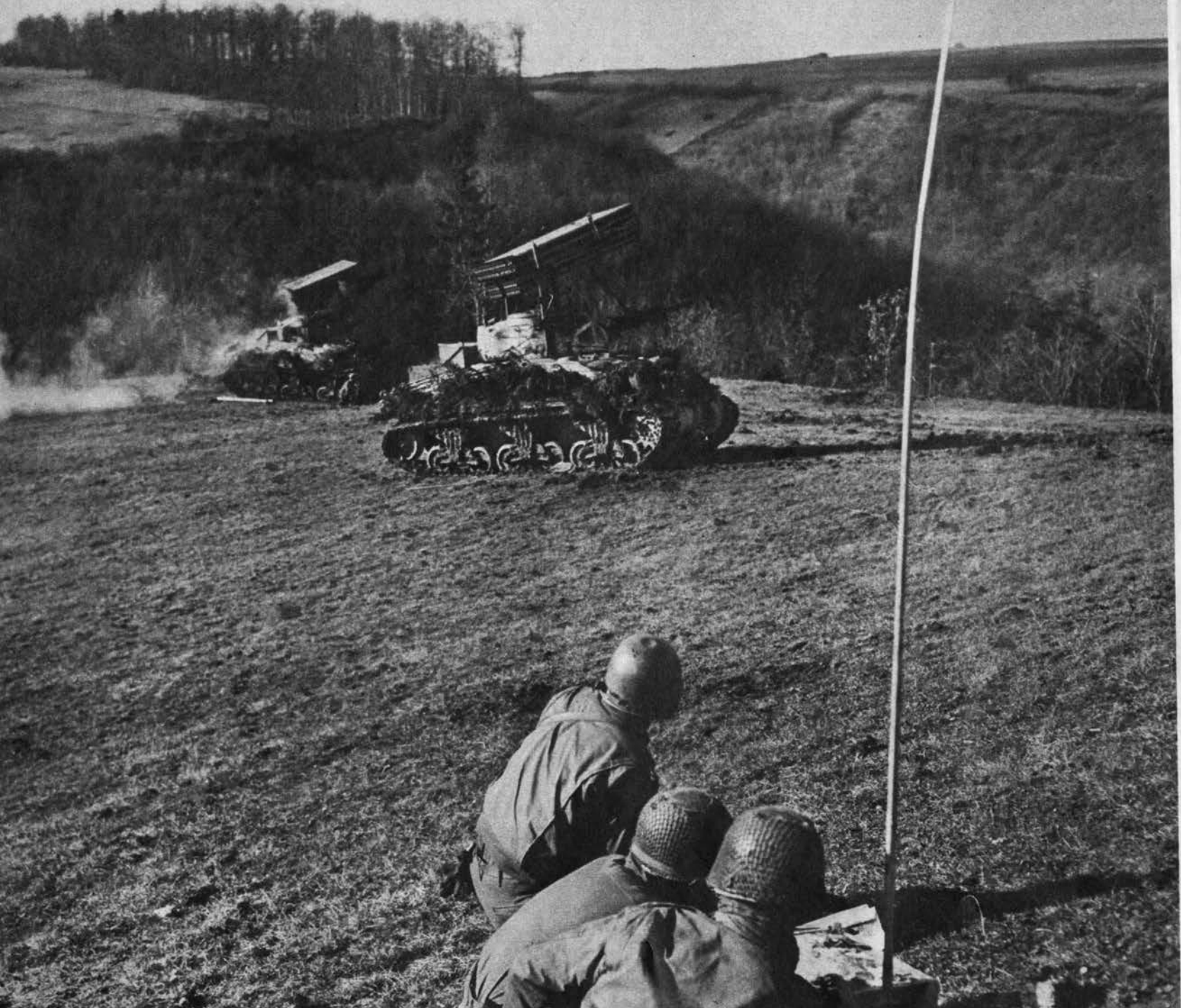
T-34 rocket launchers perch high above Sherman tank turrets as their 60 tubes guide projectiles against German positions. Supported by ver-
